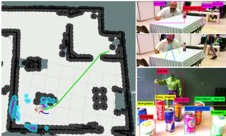
Fig. 4. LyonTech robot capabilities including navigation, people detection (Yolo), object detect (customized Yolo), pose detection (openPose)
