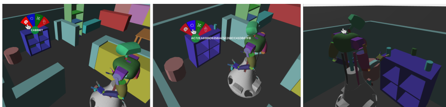
Fig. 7. Illustration of the 3D scene of the WebGUI. Users can interact with use of the menu that appears when long pressing an object in the scene. On the left figure, the user commands the robot to inspect the selected object, which is the ‘cabinet’. When the robot has inspected the ‘cabinet’, it has found entities on top of it. In the middle figure a grasp command is given to the robot to pick up an object from the cabinet. The last figure show the robot executing that action.
