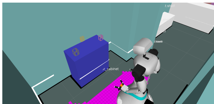
Fig. 2. A view of the world model created with ED. The figure shows the occupation grid as well as (unknown) objects recognized on top of the cabinet.
