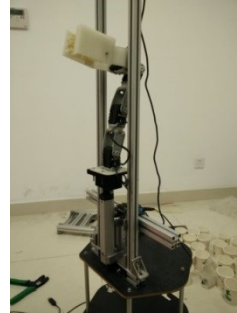
Fig. 5. Elevated arm for flexible height manipulation
