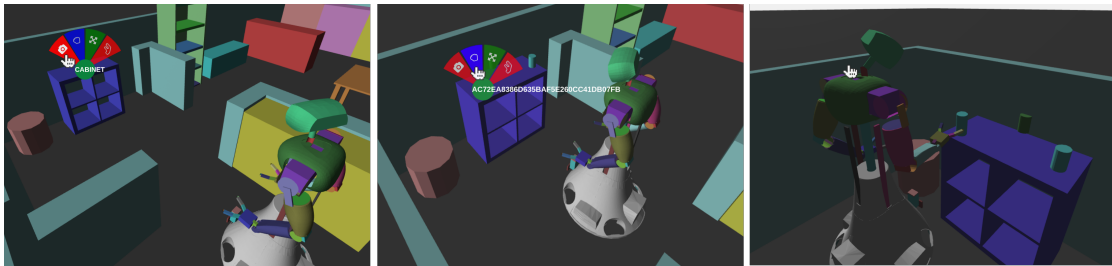
Fig. 9: Illustration of the 3D scene of the WebGUI. Users can interact with use of the menu that appears when long pressing an object in the scene. On the left figure, the user commands the robot to inspect the selected object, which is the ‘cabinet’. When the robot has inspected the ‘cabinet’, it has found entities on top of it. In the middle figure a grasp command is given to the robot to pick up an object from the cabinet. The last figure show the robot executing that action.
