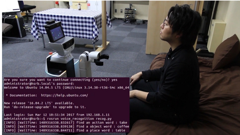
Fig. 3. Beverage delivery via speech recognition
