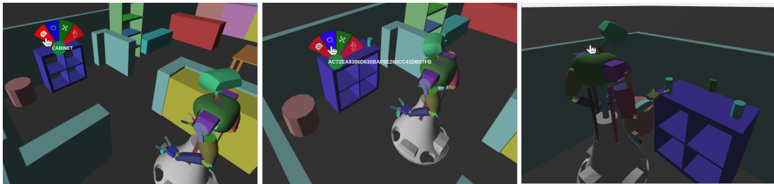
Fig. 3: Illustration of the 3D scene of the WebGUI. Users can interact with use of the menu that appears when long pressing an object in the scene. On the left figure, the user commands the robot to inspect the selected object, which is the ‘cabinet’. When the robot has inspected the ‘cabinet’, it has found entities on top of it. In the middle figure a grasp command is given to the robot to pick up an object from the cabinet. The last figure show the robot executing that action.
