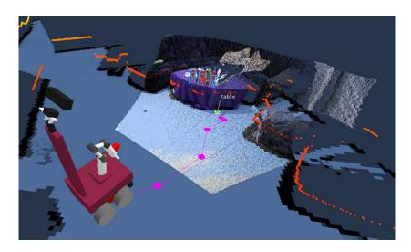
Fig. 6. Visualization of RGBD and laser sensor data. Further, a planned path to the point of interest "table" as well as grippable objects on the table are visualized.
