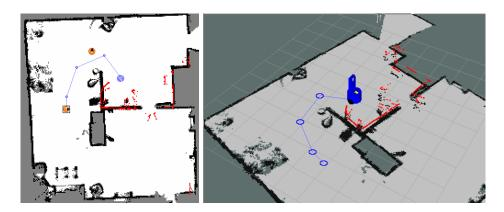
Fig. 3. 2D and 3D view of a map and a planned path (blue line). Red dots indicate the current laser scan, while orange points in the 2D map stand for navigation points.
