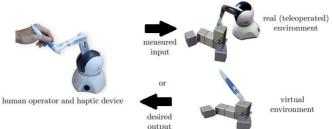
Figure 4. The haptic loop of a generic haptic interface.
