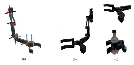
Figure 2. Bender's new arm. (a) Shows the Simulated right arm with the DOFs and the respective axes for every joint between the parts of the arm. (b) Real Right arm in a manipulation pose. (c) Different views of the real right hand gripper in a manipulate action.
