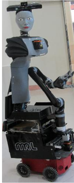
Fig. 1. Robina with Pioneer 3-AT Platform
