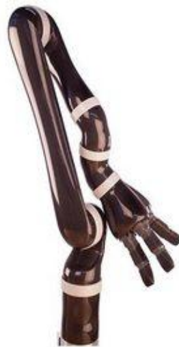
Fig. 2. Kinova Jaco Arm with 6 DOF
